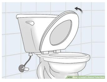
Lift your existing seat and lid to make room for the raised seat. Raised toilet seats that replace your existing seat simply sit on top of the ceramic of your toilet bowl. Most can be placed on your toilet without you needing to remove your existing seat as there's enough room between the back of the raised seat and your tank. Instead, you can simply lift the existing seat and lid up and lean it against the tank.
