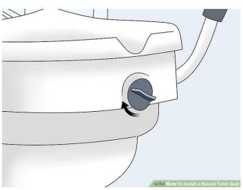
Use the adjustment knob, if required, to secure the raised seat. Some raised toilet seats have an adjustment knob at the front that's attached to an adjustment bracket inside the toilet bowl. Turn the knob counterclockwise to loosen the adjustment bracket. Turn the knob clockwise to tighten the adjustment bracket against the toilet bowl and secure it in place.
