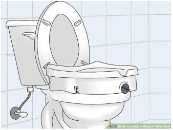
Test if the existing seat and lid can stay or needs to be removed. Place the raised toilet seat on the toilet bowl with the existing seat and lid flipped up. If there is not enough room for the existing seat and lid to sit against the tank, you'll need to remove it before you install the raised seat.
