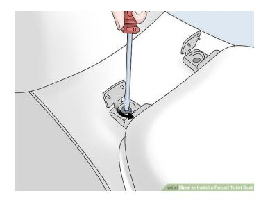
Remove your existing toilet seat if required. Kneel down in front of your toilet and reach one hand under the toilet to hold one of the nuts securing the toilet seat screw in place. Hold the nut still while using a screwdriver to loosen the screw from above. Once loose enough, remove the nut with your hand and pull out the screw. Repeat the process for the second screw and nut. Lift off the existing seat and lid and set it aside.[4]
