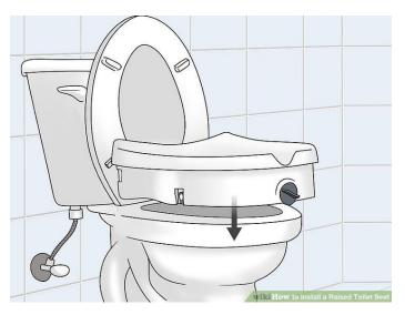
Insert the raised seat into the toilet bowl and secure the flanges. Most raised toilet seats have 1 or more flanges which hold the seat inside the toilet bowl. You may need to tilt the seat slightly forward or backwards in order to slip the flanges into the bowl. Once inserted, push the raised seat down onto the bowl until it's secured. Shake the seat gently to make sure it's been properly installed and balanced.
